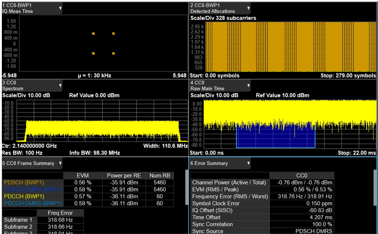
5G NR Test Mode TM1.1 100M Bandwidth 3.9G Carrier, EVM Test Value
