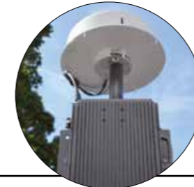
STATION CHARLIE (fixed installation): ▶ SignalShark Outdoor Unit ▶ ADFA ▶ LTE modem ▶ Software: Decodio ReX
