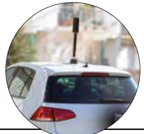
STATION ALPHA (mobile): ▶ SignalShark handheld ▶ Omnidirectional antenna ▶ LTE modem ▶ Software: Decodio ReX
