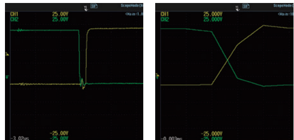
Gate signal waveforms of inverter (20 kHz) The picture on the left shows a waveforms measured with 100 MS/s (by 720211 module) that is sufficiently high sample rate to accurately reconstruct the signal, which will result in more accurate measurements than the one on the right that measured with 1 MS/s
